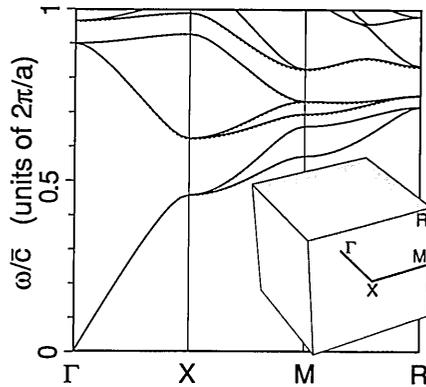
Fig. 1. Photonic band structure for close-packed air spheres in the sc lattice.  $\epsilon_b = 13$ ,  $\epsilon_a = 1$ , and  $\beta = \pi/6$ , with 750 plane waves (solid curves) by the E method. Also plotted are the lowest six bands, calculated with only 81 plane waves (overlapping dashed curves) for comparison.  $\bar{c} = c/\sqrt{\bar{\epsilon}}$ , where  $\bar{\epsilon}$  is the spatial average of  $\epsilon(\mathbf{r})$ . The inset shows the path in the sc BZ.
