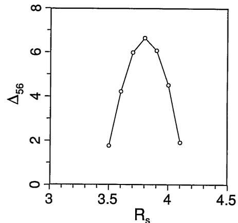
Fig. 3. Relative photonic band gap versus the radius  $R_s$  of air spheres in the sc lattice.  $\epsilon_b = 13$  and  $\epsilon_a = 1$ .  $R_s = \pi$  corresponds to the close-packed case, and at  $R_s = \pi\sqrt{2}$  the background medium becomes disconnected.
