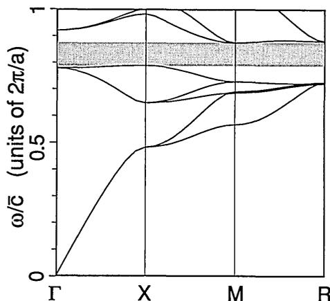
Fig. 14. Photonic band structure for the circular-air-rod structure in the sc lattice.  $\epsilon_b = 13$ ,  $\epsilon_a = 1$ , and  $\beta = 0.81$ . The radius of the air rods is  $R_c = 2.6$ .
