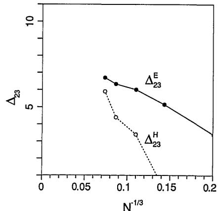
Fig. 10. Photonic band gap versus  $N^{-1/3}$  for the same structure as in Fig. 8 with the E and the H methods.
