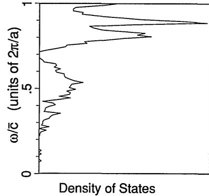
Fig. 9. Density of states computed from a random sample of 300  $\mathbf{k}$  points in the BZ for the same dielectric structure as in Fig. 8.
