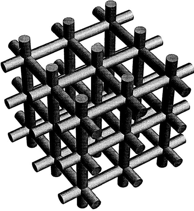
Fig. 5. Circular-rod structure. A  $3 \times 3 \times 3$  section is shown.
