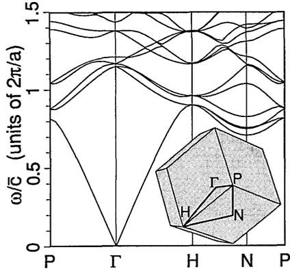
Fig. 12. Photonic bands for the scaffold structure in the bcc lattice.  $\epsilon_b = 13$ ,  $\epsilon_a = 1$ , and  $\beta = 0.84$ . 1481 plane waves were used with the E method. The H method yields the same degeneracies, but its convergence is slow.
