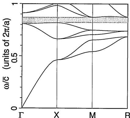
Fig. 2. Photonic band structure for overlapping air spheres in the sc lattice.  $\epsilon_b = 13$ ,  $\epsilon_a = 1$ , and  $\beta = 0.81$ . The E method was used with 750 plane waves.
