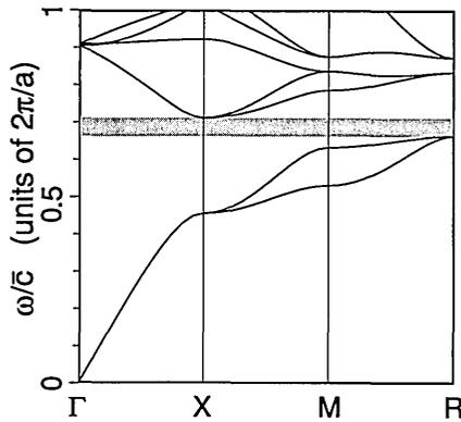
Fig. 13. Photonic band structure for the circular-dielectric-rod structure in the sc lattice.  $\epsilon_b = 1$ ,  $\epsilon_a = 13$ , and  $\beta = 0.19$ . The radius of the dielectric rods is  $R_c = 1$ .
