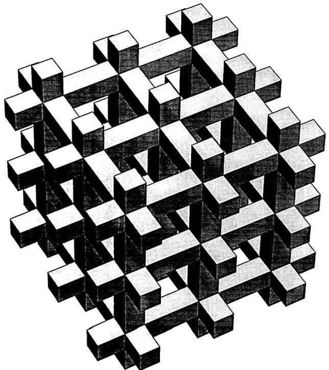
Fig. 4. Square-rod structure. A  $3 \times 3 \times 3$  section is shown.
