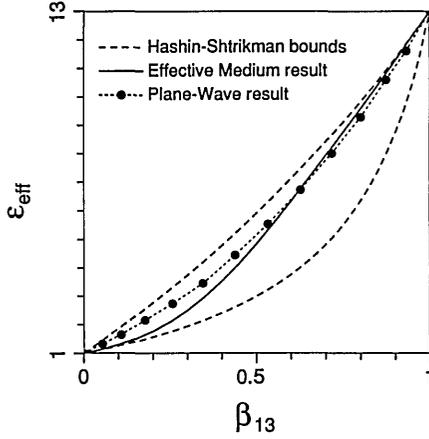
Fig. 7.  $\epsilon_{\text{eff}}$  calculated with the plane-wave method (●) for the square-rod structure in the sc lattice. Also plotted are the Hashin-Shtrikman bounds (Maxwell-Garnett results) (long dashed curves) and the effective-medium result (solid curve).  $\beta_{13}$  is the volume fraction of the  $\epsilon = 13$  material.
