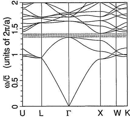
Fig. 11. Photonic bands for the same dielectric structure as in Fig. 8, calculated within the periodicity of the fcc lattice. The vertical scale is different from that of Fig. 8 because  $a_{fcc} = 2a_{sc}$ .
