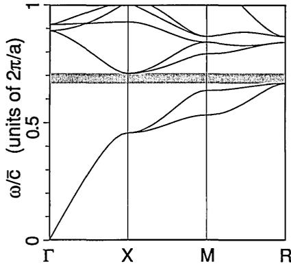
Fig. 8. Photonic bands for the square-rod structure in the sc lattice.  $\epsilon_b = 13$ ,  $\epsilon_a = 1$ , and  $\beta = 0.82$ .
